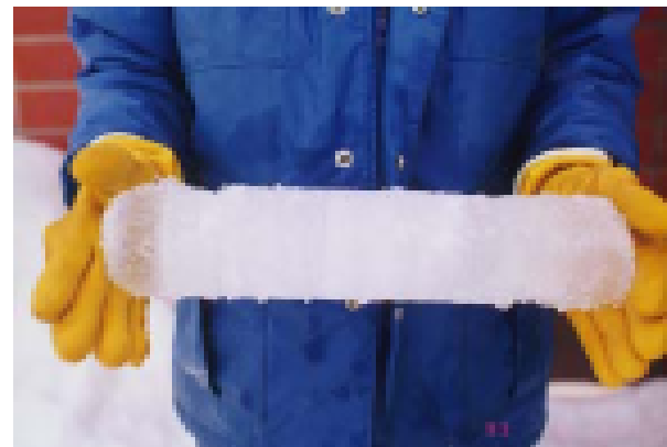
Photo 4: A core sample from the ice pond.
